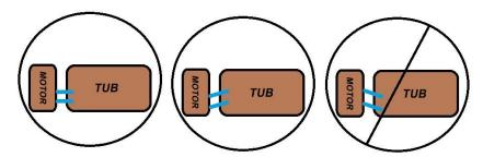
Motor unit must be level when connecting to tub or pointing up towards connections to get proper temperature readings. If motor unit is pointing down towards tub, temperature readings can be inaccurate.
