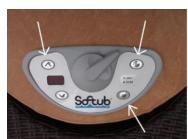
**Overnight Mode** When this mode is selected the unit will not operate for a heat call or filter cycle during the twelve hours following mode activation. This will repeat daily. When in this mode the unit will operate normally for 12 hours and standby for 12 hours. The unit must be up to the desired temperature on the LED display (ex: 104) before initializing this setting.
